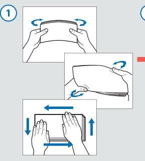
Take the stack of envelopes and loosen them, and then remove curling. Also remove the air inside the envelopes.
