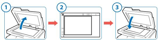
With the side of the original you want to scan face down, align the top edge of your original with the back edge of the platen glass (by the arrow in the top left corner).
